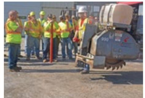
▲ Operators train on the use of a new asphalt zipper added to the Schlouch fleet.
